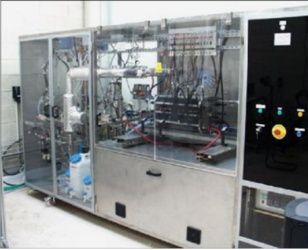
Fig. 2. Five kilowatts fuel cell test bench in the laboratory.
